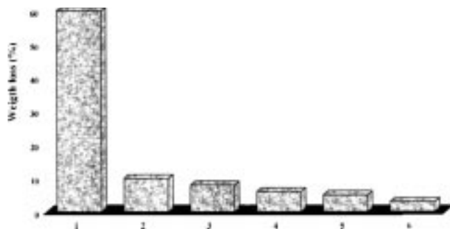
Fig. 12 Mass loss of graphite after oxidation in air at 850 °C for 4 h for different surface treatments. 1: Cg, 2: Cg (SiC), 3: Cg (SiC) + Metco 105, 4: Cg (SiC) + Metco 101, 5: Cg (SiC) + (Metco 105) enameled, and 6: Cg (SiC) + (Metco 101) enameled.
